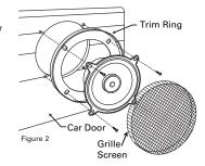
Typical installation of the Kappa i Series speakers with grilles as shown in Figure 2. NOTE: The cf Series is designed for direct replacement of factory speakers. Therefore they do not contain the grilles and trim shown in Figure 2. Installation of these models simply entails reversing the steps taken to remove the original speakers.
